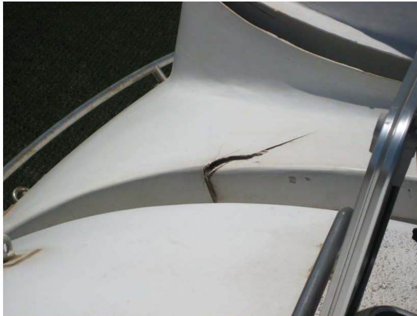
Figure 20. Structural crack near the hub of a wind turbine.
